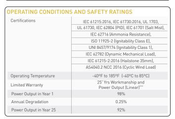
NOTE: Values at standard test conditions(STC: air mass AM1.5 irradiance 1000W/m2, temperature 25oC) based on production spread with a tolerance at Pmax, Voc & Isc. ±3% within one watt class.
